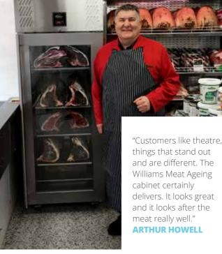
Made of stainless steel throughout, the cabinet has a capacity of 620 litres and measures 727mm wide by 889mm deep and 1960 high. It runs on eco-friendly natural refrigerant (R290) with low GWP and zero ODP. The insulation foam is precision injected, high density 80mm thick polyurethane, delivering maximum thermal properties with low GWP and zero ODP.
