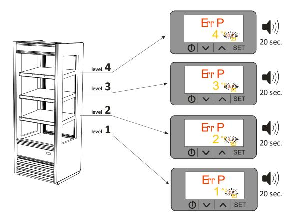
If a temperature probes failure occurs the heaters power supply is automatically switched off, a warning signal is displayed and a prolonged alarm sound is produced.
