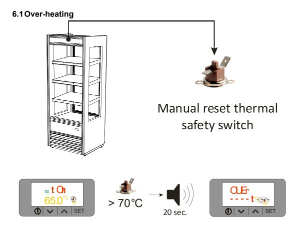
In case of regulation failure and overheating the system is protected by a manual reset switch placed behind the upper cabinet's top front.
