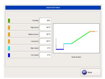
The operator can adjust the humidity and set point temperatures via this window by touching the respective parameter window.
